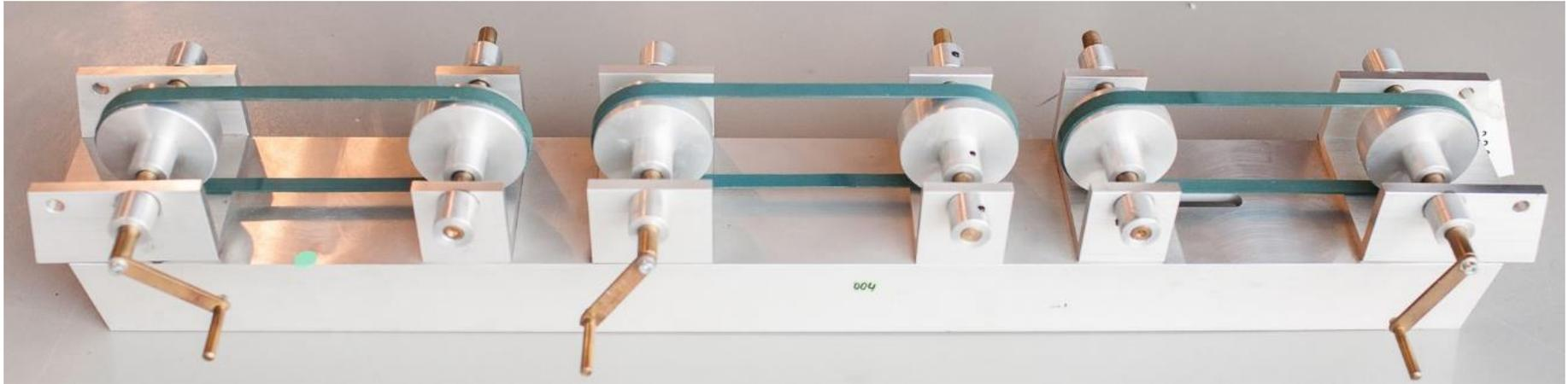
$$i = \frac{n_1}{n_2} = \frac{r_2}{r_1} \cdot \frac{1}{1-s} \leq \frac{r_2}{r_1}$$
